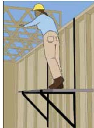
scaffolds or ladders for floor joist installation and decking.
